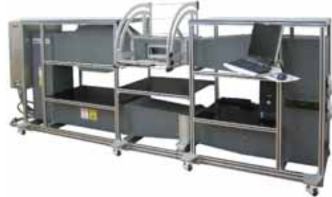
Fig. C: FDK Original Wind Tunnel
