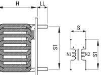
General InformationSeriesSC-JHStyleThrough-HoleRoHSYesNotesLead Spacing (S/S1) Are For Reference Only.MiscellaneousTemperature Rise Maximum: 80 K.CoreMn-Zn Ferrite
