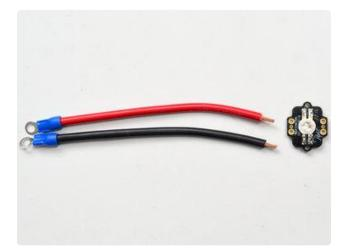
For the power wires, make sure to get nice hefty ones that can handle the current draw. Of course, it matters how long they're going to be, and how many Pixies are in the chain, and how much they will be lit up. 16 AWG is the recommended size.
