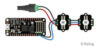
Feather TX to Pixie data in Feather Gnd to Pixie shared ground Pixies require an external power source and sufficient gauge power wire! Follow the previous pages in this guide to ensure you have wired them properly.
