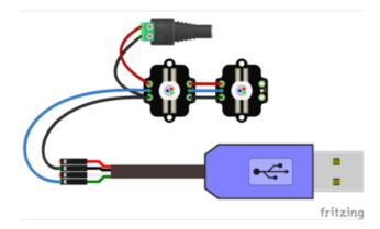
USB serial TX to Pixie data in USB serial ground to Pixie shared ground Pixies require an external power source and sufficient gauge power wire! Follow the previous pages in this guide to ensure you have wired them properly.
