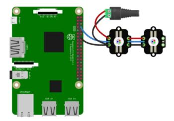
Pi TX to Pixie data in Pi Gnd to Pixie shared ground Pixies require an external power source and sufficient gauge power wire! Follow the previous pages in this guide to ensure you have wired them properly.
