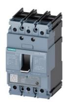
circuit breaker 3VA5 UL frame 125 breaking capacity class H 65kA @ 480 V 3-pole, line protection TM230, FTAM, In=125A overload protection Ir=125A fixed short-circuit protection Ii=5...10 x In cable connection on both sides
