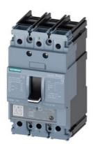
circuit breaker 3VA5 UL frame 125 breaking capacity class M 35kA @ 480 V 3-pole, line protection TM230, FTAM, In=30A overload protection Ir=30A fixed short-circuit protection li=5...10 x In cable connection on both sides
