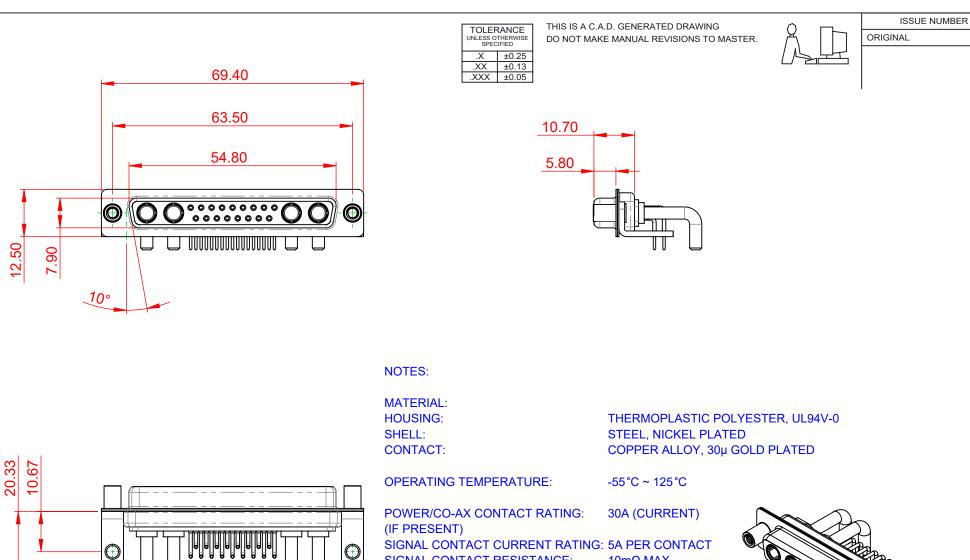
SIGNAL CONTACT RESISTANCE:  $10m\Omega$  MAX.
