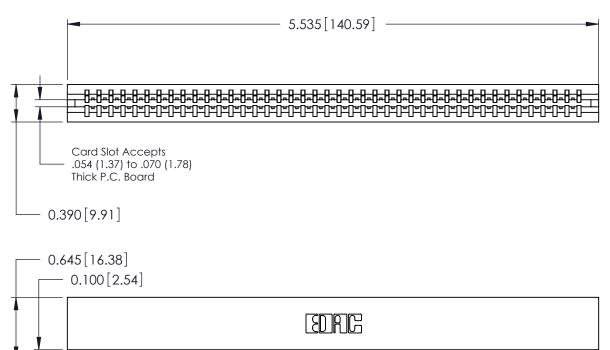
746 Series Ultra-Mate Card Edge Connector - Press Fit Part Number: 746-042-527-506
