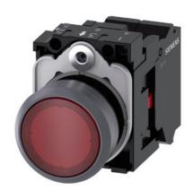
Illuminated pushbutton, 22 mm, round, plastic with metal front ring, red, pushbutton, flat, momentary contact type, with holder, 1NC, LED module with integrated LED 24 V AC/DC, spring-type terminal, with laser labeling, upper case
