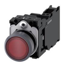
Illuminated pushbutton, 22 mm, round, plastic with metal front ring, red, pushbutton, flat, momentary contact type, with holder, 1 NO+1 NC, LED module with integrated LED 24 V AC/DC, spring-type terminal, with laser labeling, inscription or symbol Customer-specific selection with SIRIUS ACT configurator (CIN)
