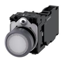
Illuminated pushbutton, 22 mm, round, plastic with metal front ring, white, pushbutton, flat, momentary contact type, with holder, 1 NO+1 NC, LED module with integrated LED 24 V AC/DC, screw terminal, with laser labeling, lower case
