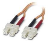
Assembled FO cable, zip cord cable, multi-mode fiberglass 50/125 µm, OM2, plug: SC duplex/SC duplex, degree of protection: IP20, for installation in cable ducts or control cabinets, length: 1 m
