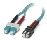
Assembled FO cable, zip cord cable, multi-mode fiberglass 50/125 µm, OM3, plug: SC duplex/SC-RJ, degree of protection: IP20, for installation in cable ducts or control cabinets, length: 1 m
