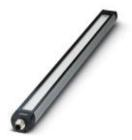
LED machine light, 24 V DC, emission angle 40 °/80 °, color temperature 5000 K, length 540 mm, diameter 40 mm, M12 connector, Light housing: Anodized aluminum, Pane: Single-pane safety glass (ESG, thermally toughened float glass), pivoting, resistant to coolants and lubricants
