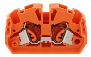
Feed-through terminal for direct mount, Tension-spring connection, Mounting type: Mounting surface, Rated cross-section: 2.5 mm<sup>2</sup>, Width: 11.1 mm, Colour: Orange
