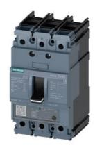
circuit breaker 3VA5 UL frame 125 breaking capacity class S 25kA @ 480 V 3-pole, line protection TM230, FTAM, In=35A overload protection Ir=35A fixed short-circuit protection Ii=5...10 x In nut keeper kit on both sides
