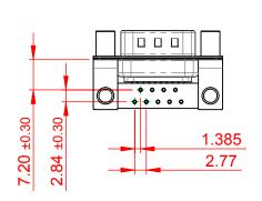
THIS IS A C.A.D. GENERATED DRAWING TOLERANCE UNLESS OTHERWISE SPECIFIED DO NOT MAKE MANUAL REVISIONS TO MASTER. .X ±0.25 .XX ±0.13 .XXX ±0.10
