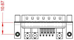
50Ω (IMPEDANCE) POWER/CO-AX CONTACT RATING: (IF PRESENT) SIGNAL CONTACT CURRENT RATING: 5A PER CONTACT SIGNAL CONTACT RESISTANCE:  $10m\Omega$  MAX. **INSULATOR RESISTANCE:**
