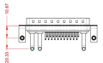
POWER/CO-AX CONTACT RATING:30A (CURRENT)(IF PRESENT)SIGNAL CONTACT CURRENT RATING:5A PER CONTACTSIGNAL CONTACT RESISTANCE:10mΩ MAX.INSULATOR RESISTANCE:5000MΩ min.DIELECTRIC5000MΩ min.
