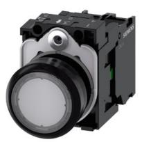
Illuminated pushbutton, 22 mm, round, plastic, clear, pushbutton, flat, momentary contact type, with holder, 1NO, LED module with integrated LED 24 V AC/DC, screw terminal, Z=20-unit packaging
