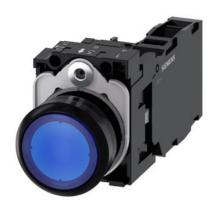
Illuminated pushbutton, 22 mm, round, plastic, blue, pushbutton, flat, momentary contact type, with holder, 1 NO+1 NC, LED module with integrated LED 110 V AC, screw terminal, with laser labeling, inscription or symbol Customer-specific selection with SIRIUS ACT configurator (CIN)
