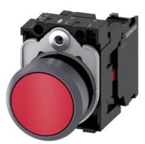
Pushbutton, 22 mm, round, plastic with metal front ring, red, pushbutton, flat, momentary contact type, with holder, 1 NC, screw terminal, with laser labeling, upper case and lower case, always upper case at beginning of line
