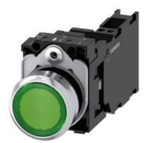
Illuminated pushbutton, 22 mm, round, metal, shiny, green, pushbutton, flat, momentary contact type, with holder, 1 NO+1 NC, LED module with integrated LED 110 V AC, spring-type terminal, with laser labeling, upper case and lower case, Always upper case at the beginning of the word
