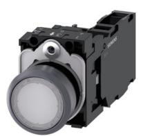
Illuminated pushbutton, 22 mm, round, plastic with metal front ring, white, pushbutton, flat, momentary contact type, with holder, 1 NO+1 NC, LED module with integrated LED 110 V AC, screw terminal, with laser labeling, upper case and lower case, always upper case at beginning of line
