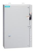
Non-reversing motor starter, Size 1, Three phase full voltage, Solid-state overload relay, OLR amp range 0.25-1A, 24VAC 50-60Hz coil, Combination type, 30A fusible disconnect, 30A/250V fuse clip, Enclosure NEMA type 4/12, Water/dust tight for outdoors, Extra-wide enclosure
