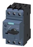
Circuit breaker size S0 For transformer protection A-release 2.2...3.2 A Short-circuit release 65 A Screw terminal Standard switching capacity
