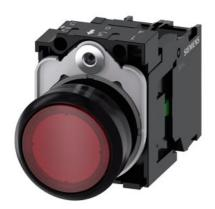
Illuminated pushbutton, 22 mm, round, plastic, red, pushbutton, flat, momentary contact type, with holder, 1NO, LED module with integrated LED 24 V AC/DC, screw terminal, with laser labeling, upper case and lower case, Always upper case at the beginning of the word
