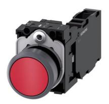
Pushbutton, 22 mm, round, plastic with metal front ring, red, pushbutton, flat, momentary contact type, with holder, 1 NO+1 NC, screw terminal, with laser labeling, inscription or symbol Customer-specific selection with SIRIUS ACT configurator (CIN)
