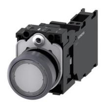
Illuminated pushbutton, 22 mm, round, plastic with metal front ring, clear, pushbutton, flat, momentary contact type, with holder, 1 NO+1 NC, LED module with integrated LED 24 V AC/DC, spring-type terminal, with laser labeling, lower case
