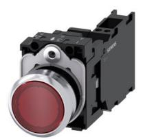
Illuminated pushbutton, 22 mm, round, metal, shiny, red, pushbutton, flat, momentary contact type, with holder, 1 NO+1 NC, LED module with integrated LED 24 V AC/DC, spring-type terminal, with laser labeling, upper case and lower case, always upper case at beginning of line
