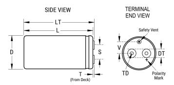
General Information Series ALS70 Dielectric Aluminum Electrolytic Description Screw Terminal, Aluminum Electrolytic RoHS AEC-Q200 No Halogen Free Yes Component 75 g Weight Dimensions D And L Include Sleeving. MS (MxH) = Notes M8x12. Mounting Clamp (Sold Separately): V3/H2/2736 Shelf Life 156 Weeks
