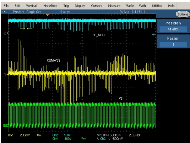
Figure 27. During startup when the current is high, COM-VSS noise is high (yellow), fault conditions occur (blue), compressor will eventually stall, 2ms/div
