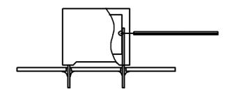
Temperature monitored inside the capacitor.
