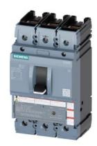
circuit breaker 3VA5 UL frame 250 breaking capacity class C 100kA @ 480 V 3-pole, line protection TM230, FTAM, In=200A overload protection Ir=200A fixed short-circuit protection Ii=5...10 x In UL489 SB (naval), 50 deg. cel. cable connection on both sides
