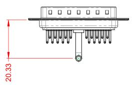
30A (CURRENT) POWER/CO-AX CONTACT RATING: (IF PRESENT) SIGNAL CONTACT CURRENT RATING: 5A PER CONTACT SIGNAL CONTACT RESISTANCE:  $10m\Omega$  MAX. INSULATOR RESISTANCE:
