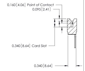
ACAD REFERENCE NO. 746 Series Ultra-Mate Card Edge Connector - Press Fit DRAWN: Part Number: 746-038-545-506 CHECKED: **EDAC INC** THESE DRAWINGS AND SPECIFICATIONS ARE THE PROPERTY OF EDAC INC.,AND TORONTO, ONTARIO SHALL NOT BE REPRODUCED, OR COPIED CANADA OR USED AS THE BASIS FOR THE
