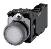
Illuminated pushbutton, 22 mm, round, plastic with metal front ring, white, pushbutton, flat, momentary contact type, with holder, 1 NO+1 NC, LED module with integrated LED 230 V AC, screw terminal, with laser labeling, upper case and lower case, Always upper case at the beginning of the word
