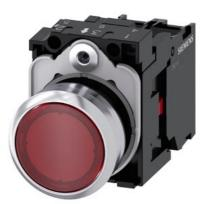
Illuminated pushbutton, 22 mm, round, metal, shiny, red, pushbutton, flat, momentary contact type, with holder, 1NC, LED module with integrated LED 230 V AC, screw terminal, with laser labeling, symbol number according to, ISO 7000 or IEC 60417
