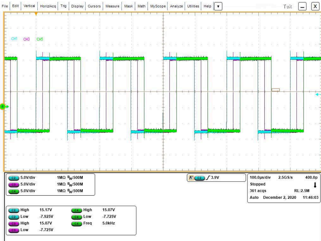
Figure 3-2. Gate Waveforms for Driver Channels Ch1, Ch3, Ch5
