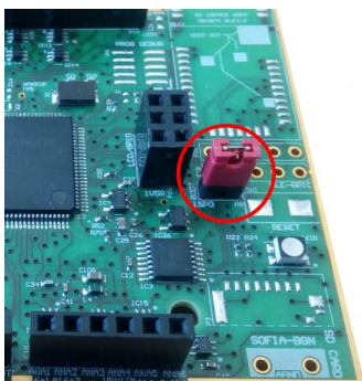
Figure 41. Position of the BOOT Pins
