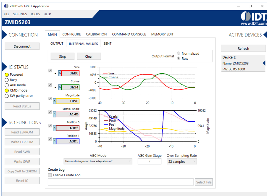
Figure 9. “INTERNAL VALUES” Tab – ZMID5203 Example
