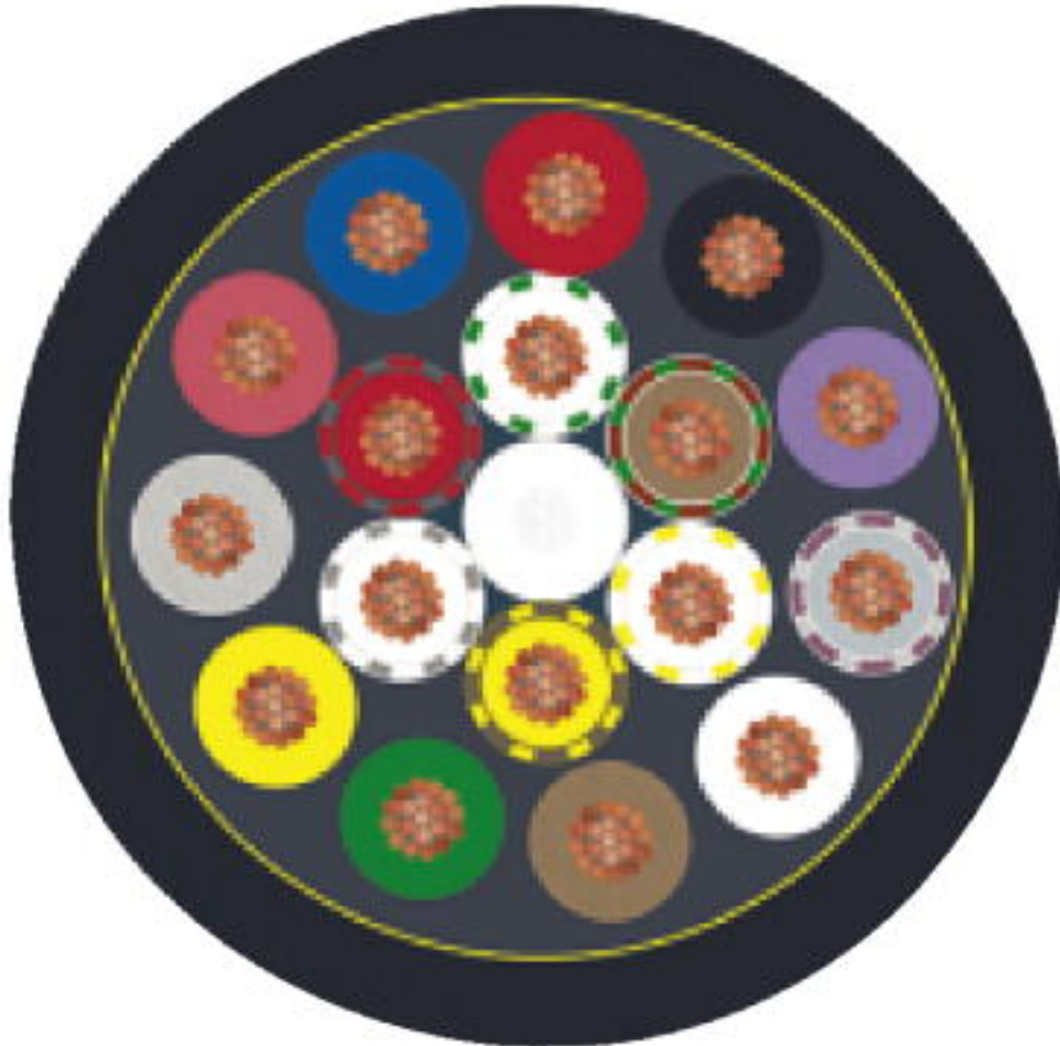
Cable cross section
