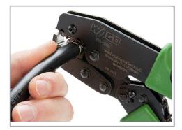
Squeeze handles until ratchet mechanism is released.
