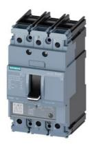
circuit breaker 3VA5 UL frame 125 breaking capacity class S 25kA @ 480 V 3-pole, line protection TM230, FTAM, In=110A overload protection Ir=110A fixed short-circuit protection Ii=5...10 x In UL489 SB (naval), 50 deg. cel. cable connection on both sides
