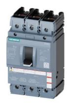
molded case switch 3VA5 UL frame 250 max. sh-circ breaking capacity 100kA @ 480 V 3-pole, line protection MCS110, In=150A without overload protection self-protection Ii=16 x In cable connection on both sides
