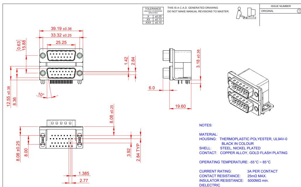
WITHSTANDING VOLTAGE: 1000V AC rms
