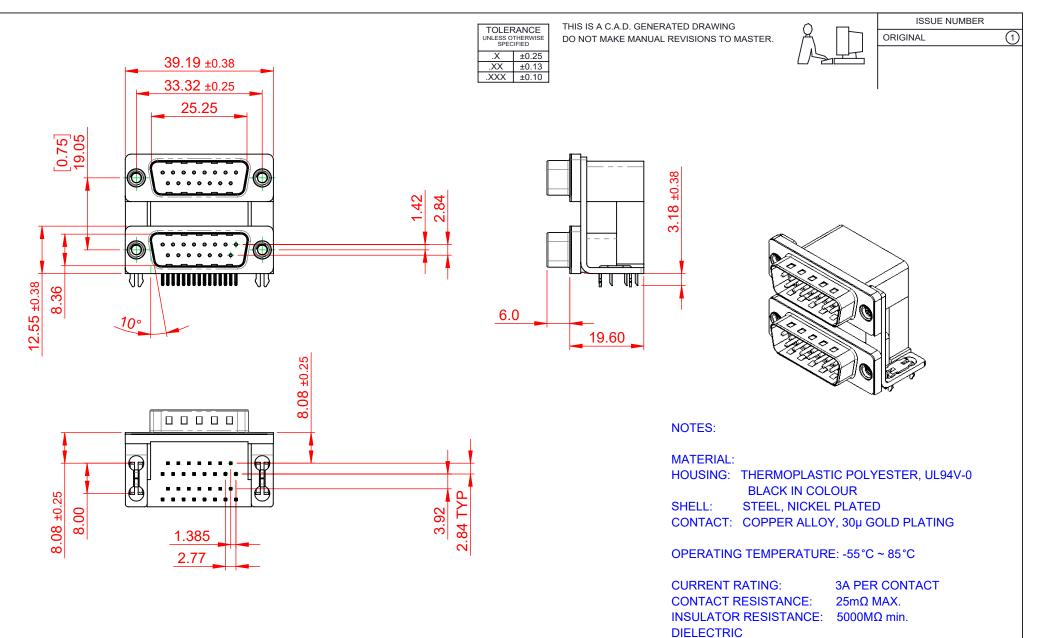
WITHSTANDING VOLTAGE: 1000V AC rms
