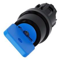
Key-operated switch O.M.R, 22 mm, round, plastic, lock number 73038, blue, with 2 keys, 2 switch positions O-I, latching, actuating angle 90°, 10:30h/13:30h, key removal O+I, with laser labeling, lower case
