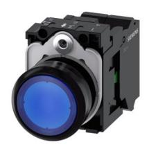
Illuminated pushbutton, 22 mm, round, plastic, blue, pushbutton, flat, momentary contact type, with holder, 1NO, LED module with integrated LED 24 V AC/DC, spring-type terminal, with laser labeling, upper case and lower case, Always upper case at the beginning of the word
