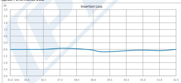
Click the following link (or enter part number in "SEARCH" on website) to obtain additional part information including price, inventory and certifications: Isolator with 14 dB Isolation from 35 GHz to 42.5 GHz, 10 Watts and 2.4mm Female PE83IR1038
