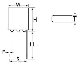
Series T340 Dielectric MnO2 Tantalum Style Radial Molded Radial, Solid Tantalum, Molded Description RoHS Yes Termination Tin AEC-Q200 No Molded Construction Includes Standoff Height of 0.38 +/- 0.13mm. Miscellaneous Longest Lead Is Positive. Notes
