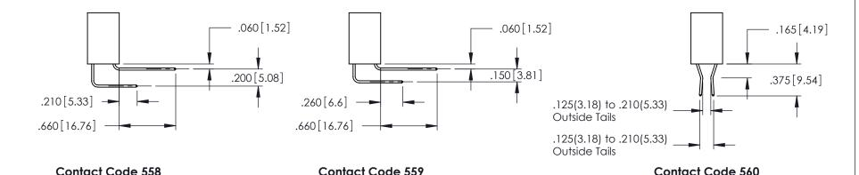
INSULATOR MATERIAL: THERMOPLASTIC POLYESTER, UL 94V-0 CONTACT MATERIAL; COPPER, NICKEL, TIN ALLOY CA-725 CONTACT PLATING: GOLD ON THE MATING AREA, TIN-LEAD
